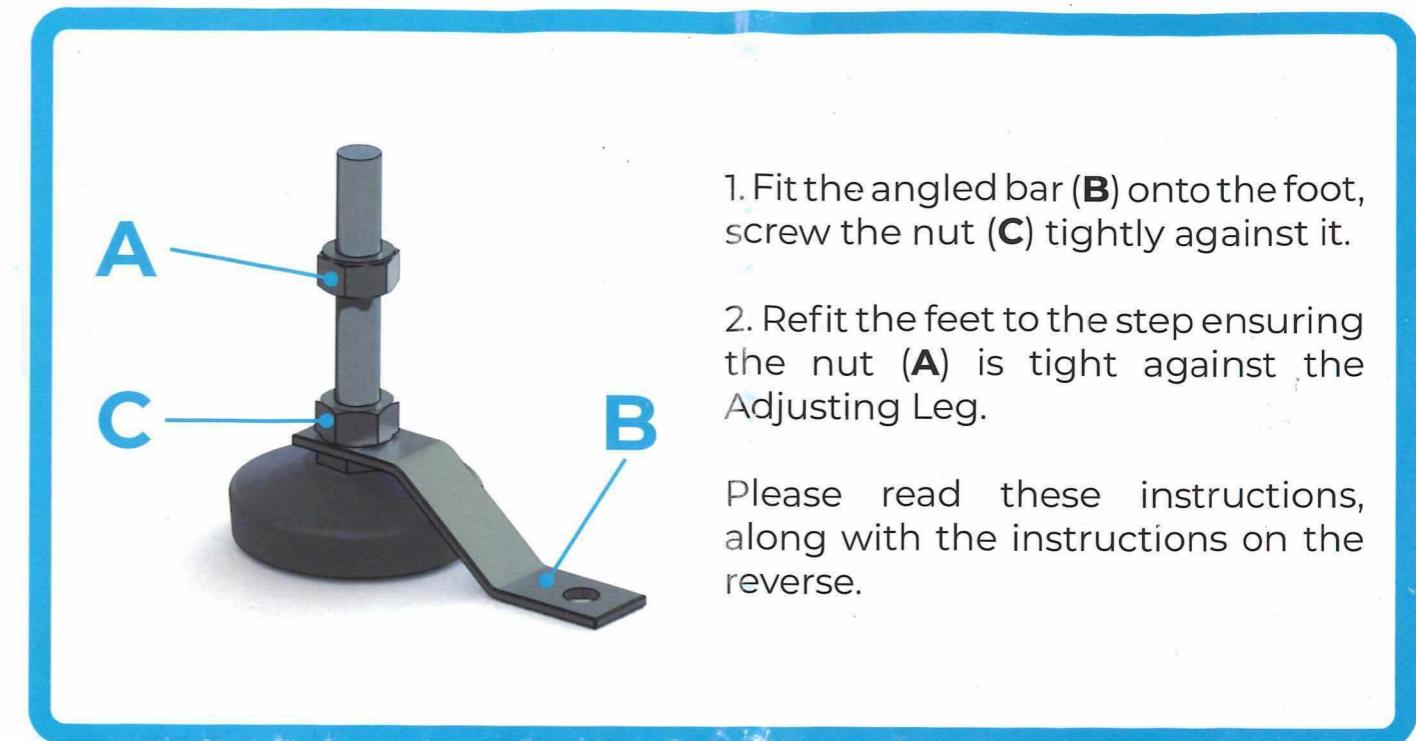
1. Fit the angled bar (**B**) onto the foot, screw the nut (**C**) tightly against it.
